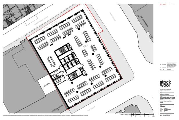
Proposed - Typical office floor plan (1<sup>st</sup> to 4<sup>th</sup> floor)
